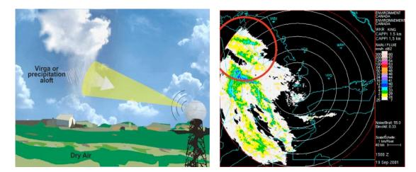
Radar detecting precipitation, that is occurring aloft, but not reaching the ground.
