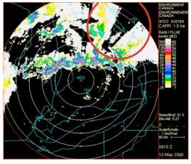
Storms closest to radar reflect or absorb most of the available radar energy leaving reduced amount of energy to detect more distant storms.
