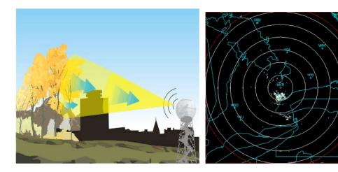
Note - the radar beam lobe, and the fact that the lobe does not extend immediately overhead of the site.
